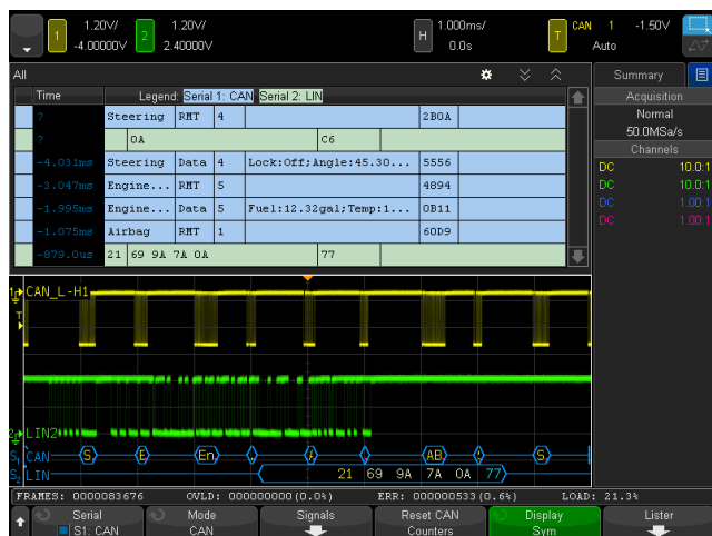
Figure 6: Dual time-interleaved lister display makes it easier to track data through CAN-to-LIN gateways.
